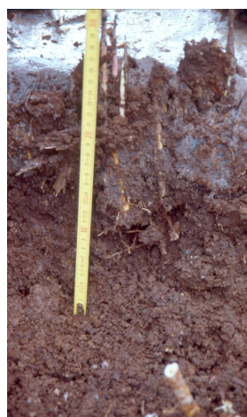
Figure 2.13: Deposit layer of Gensac la Pallue (France) 1st stage filter (dredging in 2001).
