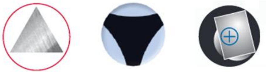
Figure 5 : section des limes RaCe®, ProFile® et ProTaper Next® (22, 23, 24).
